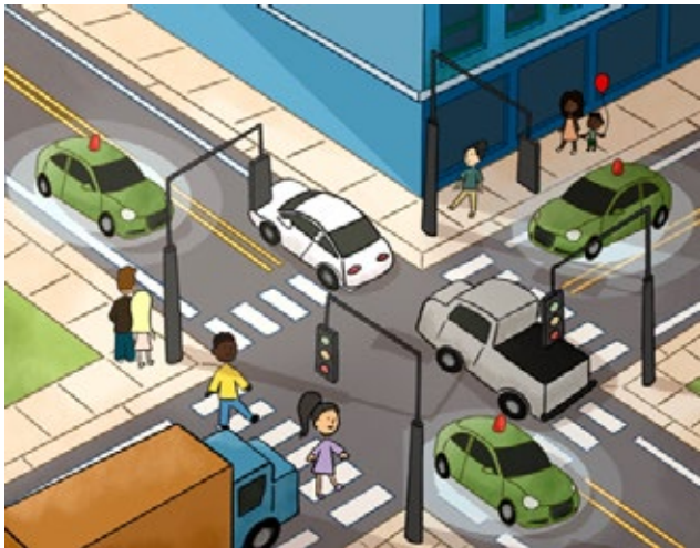
CAVs and HDVs approaching a signalized intersection with V2I and V2V communications.
