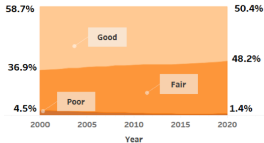
Figure 1. Percentage of Texas statewide bridge deck area in good, fair, and poor condition over the past 20 years.
