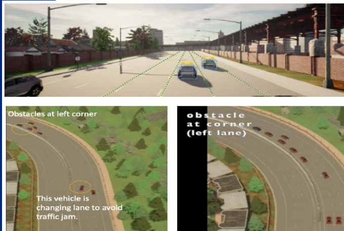
Figure 1. traffic environment developed in CARLA showed urban setup, multiple lanes of a road, traffic signs, and multiple vehicles in motion. (Upper) A controlled vehicle changes its lane to avoid the traffic jam with information sharing. (Bottom Left) Traffic jam on the left lane without route redirection and information sharing with more vehicles taking the left lane. (Bottom right)
