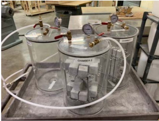
Figure 1. Sulfate impregnation chamber prior to introducing sulfate solution.
