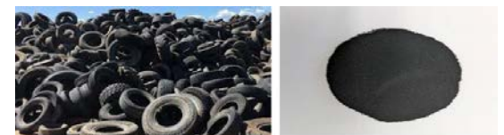
Figure 1. (a) Stockpiled Waste Tires in a Landfill and (b) Processed GTR Sample (Mesh #40).
