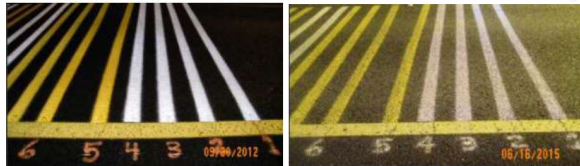
Figure 1: White and yellow markings after installation (left) and after 36 months (right) for one of markings installed in Florida.
