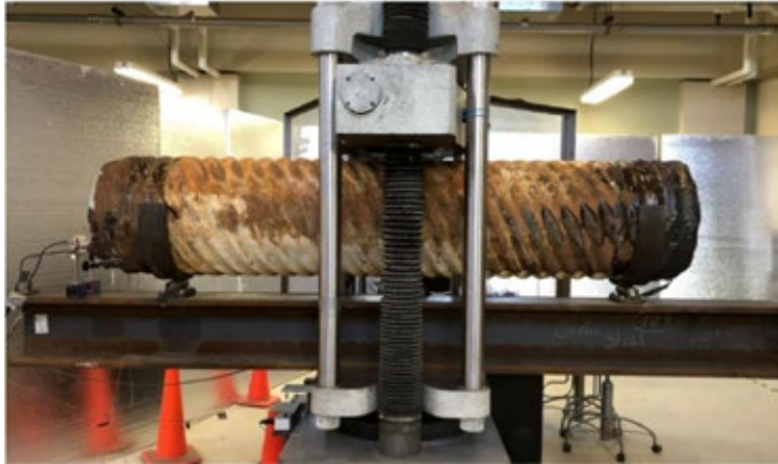
Experimental set-up for testing corroded CMP retrofitted with GFRP profile liner under three-point bending.
