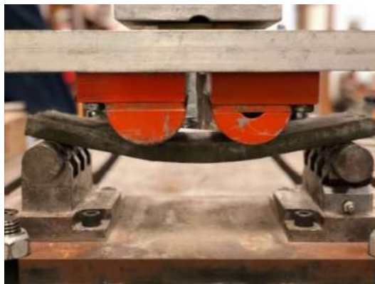
Figure 1: Ductile Behavior of ECC Material Developed at LSU
