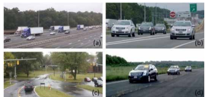
Examples of mobility-based CAV applications: (a) truck platooning, (b) cooperative merging, (c) signalized intersection approach and departure, and (d) CACC.
