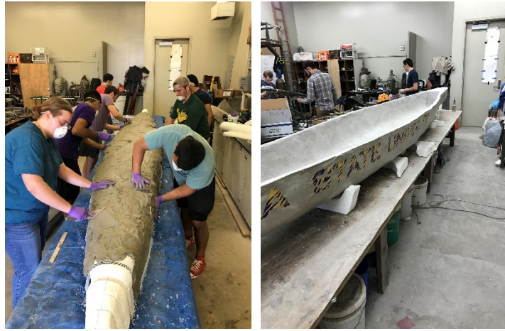
Figure 3: ASCE Concrete Canoe Competition (a) Students Manufacturing the Concrete Canoe with Lightweight Cost-Effective ECC-like Material (b) Finalized Concrete Canoe
