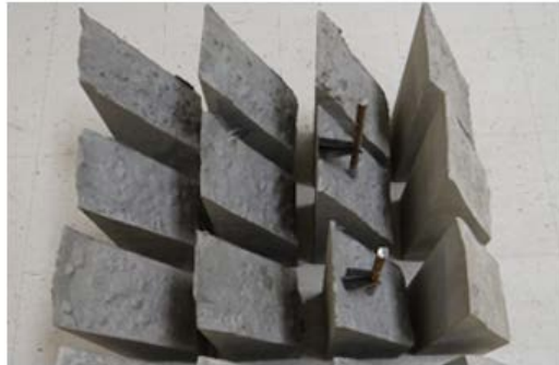
Figure 2. Slant shear specimens under preparation.
