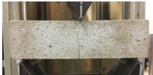
Figure 1. Crack propagation in concrete beam under three-point bending.
