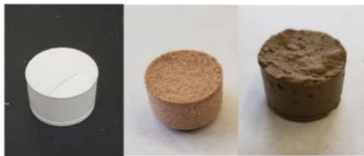
Figure 2. Pure geopolymer (left) sample and samples of sand (middle) and soil (right) stabilized with 10% geopolymers (by volume) after curing.
