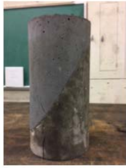
Figure 2. Split cylinder sample and stress state induced during compression test.
