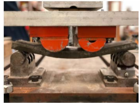
Figure 2. ECC during a Flexural Test.
