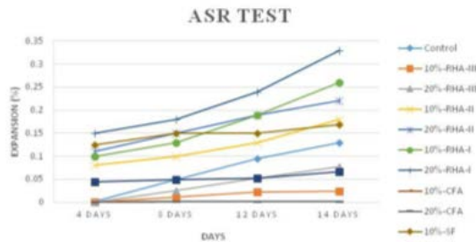
Figure 2. Effect of ASR expansion on RHA, CFA and SF modified concrete.
