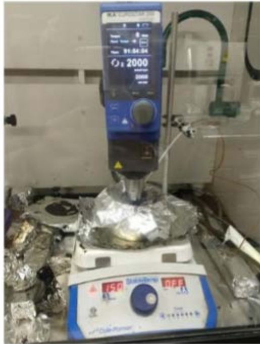
Figure 1. High Shear Mixer Used for Blending.
