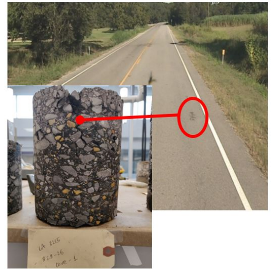
Figure 2. Successful identification of top-down cracking using digital image analysis
