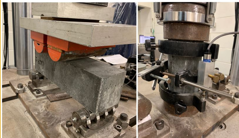
Figure 2. Set-up for cracking beams, prior to monitoring self-healing (left); Set-up for the modulus of elasticity test, to be conducted before and after healing (right).
