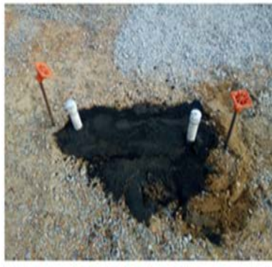
Figure 2. Field demonstration on RHA modified flowable fill concrete.
