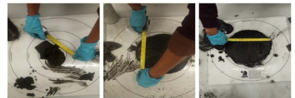
Figure 1. Trial mix of FFC with different w/c ratios (from left: 2.0 w/c, 2.5 w/c, 2.7 w/c, respectively).
