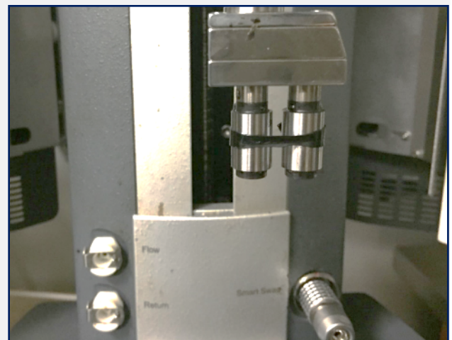
Asphalt binder sample during an extensional deformation test
