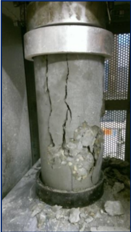
Compressive strength test of RHA specimen
