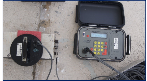
In-situ measurements of exposed RC sample using a ring probe
