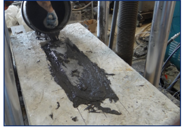
Preparing test specimen to replicate pavement repair with UHP-FRC concrete
