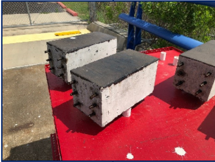
Exposed RC samples being monitored in Galveston, TX
