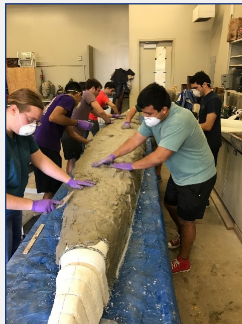
ASCE students casting the fiber reinforced concrete to form their canoe
