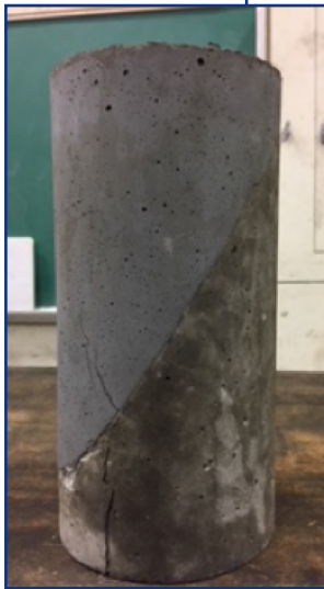
Split cylinder sample for compression test
