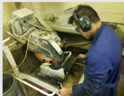
Preparing asphalt samples for testing
